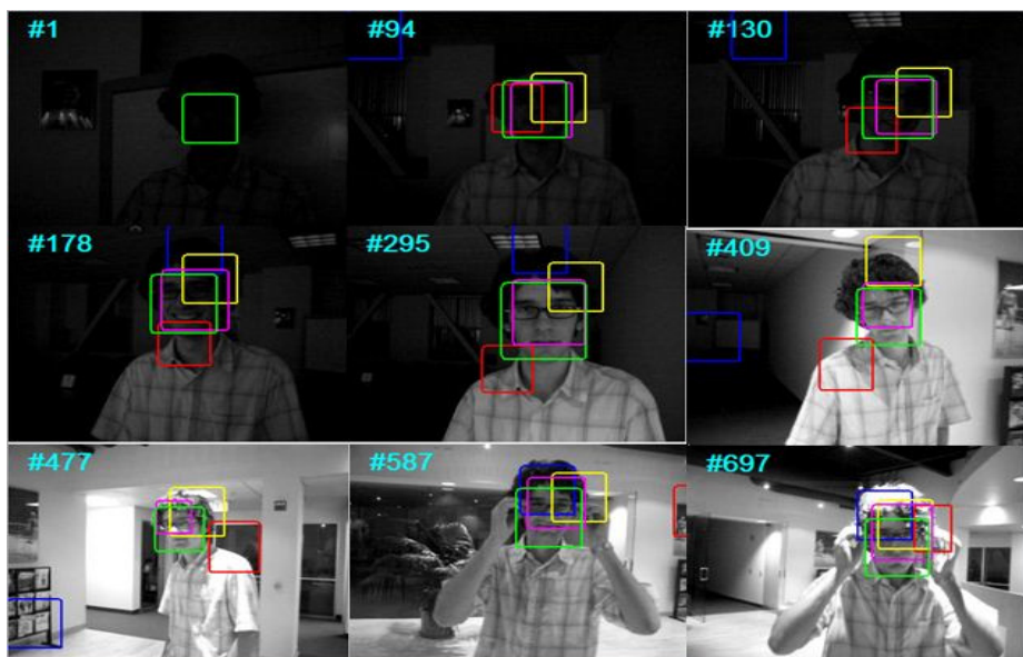
Fig. 2. Representative frames on sequences David under illumination changes. Blue, red, yellow, magenta and green bounding boxes were generated by FT, L1, MIL, TLD, and ours, respectively.
