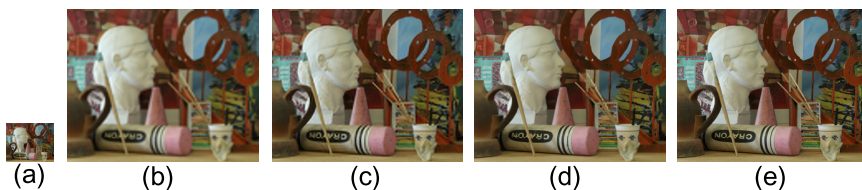
Fig. 4. Super-resolution results of Art (view 2) with a scale factor 4. (a), the low-resolution input. (b), result of bicubic interpolation method. (c), result of sparse coding method. (d), result of proposed method. (e) the groundtruth.
