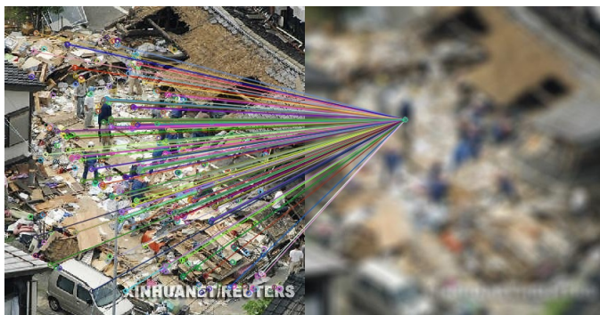
Fig. 1. One mismatch example using ORB, almost all the candidate points in the left image are matched with the same one point in the right one
