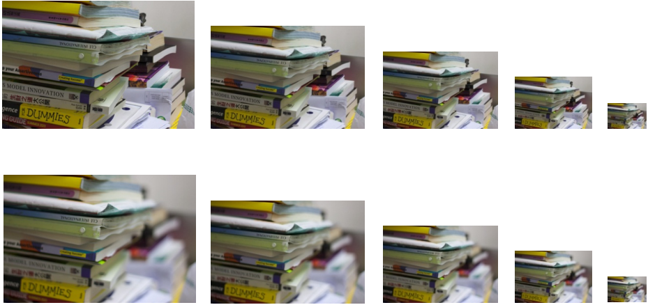
Fig. 4. As the image pair becomes smaller and smaller, overall, I_A (top row) and I_B (bottom row) will become more and more similar to each other. While sharp areas in both images will always stay similar to each other, areas that are sharp in I_A but blurred I_B in will not appear similar until they are shrunk to relatively small dimensions.
