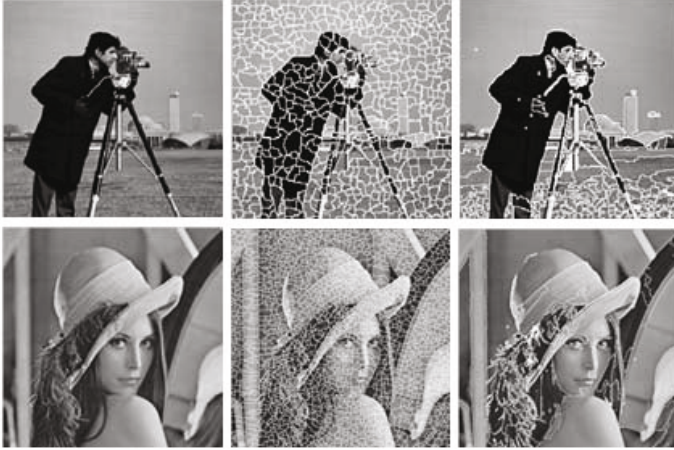
Fig. 1. Pre-segmentation comparison of watershed and mean shift with a boundary confidence prior algorithm
