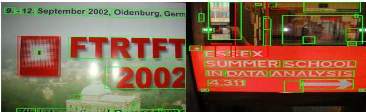
Fig. 4. The SWT results combined with CCA and MMF. The green boxes are the textual candidate regions, and the red regions are filtered by CCA and MMF.
