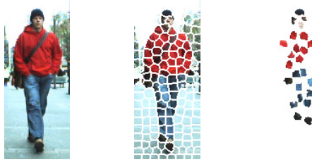
Fig. 2. An example of super pixel segmentation result. From left to right: original image, image segmented, visual patches generated by segmentation.
