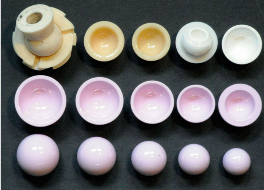
Fig. 1.1 The three generations of ceramics used in hip arthroplasty as bearing materials: ( top left to bottom right ) first-generation BIOLOX® threaded cup Ø 38 mm, second-generation BIOLOX® forte Ø 28 mm ( thick and thin inlay ), third-generation ceramys® Ø 28 mm ( thick and thin inlay ), BIOLOX® delta Ø 44, 40, 36, 32, 28 mm
