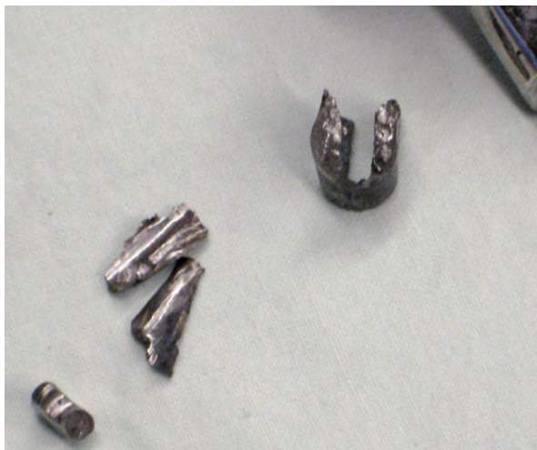
Fig. 16.3 Remnants of fractured neck left within morse taper requiring removal with midas rex
