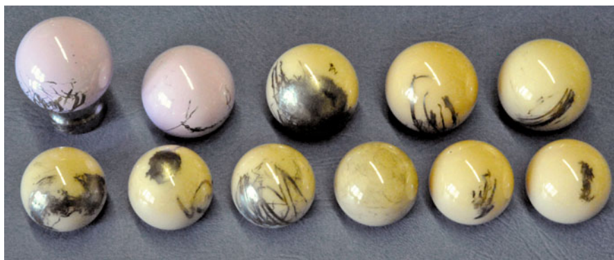
Fig. 1.8 Examples for metal transfer to ceramic heads (Courtesy of Hartmut Kiefer)
