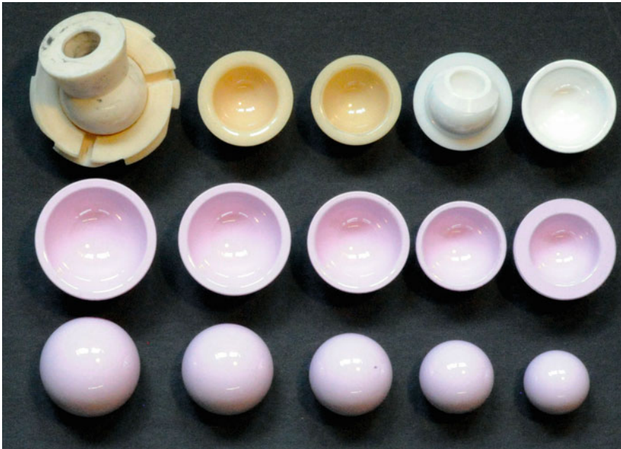
Fig. 1.1 The three generations of ceramics used in hip arthroplasty as bearing materials: ( top left to bottom right ) first-generation BIOLOX® threaded cup Ø 38 mm, second-generation BIOLOX® forte Ø 28 mm ( thick and thin inlay ), third-generation ceramys® Ø 28 mm ( thick and thin inlay ), BIOLOX® delta Ø 44, 40, 36, 32, 28 mm
