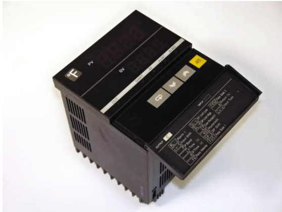
Fig. 88.1. Omron™ E5AF: An industrial fuzzy controller of the early 1990’s
