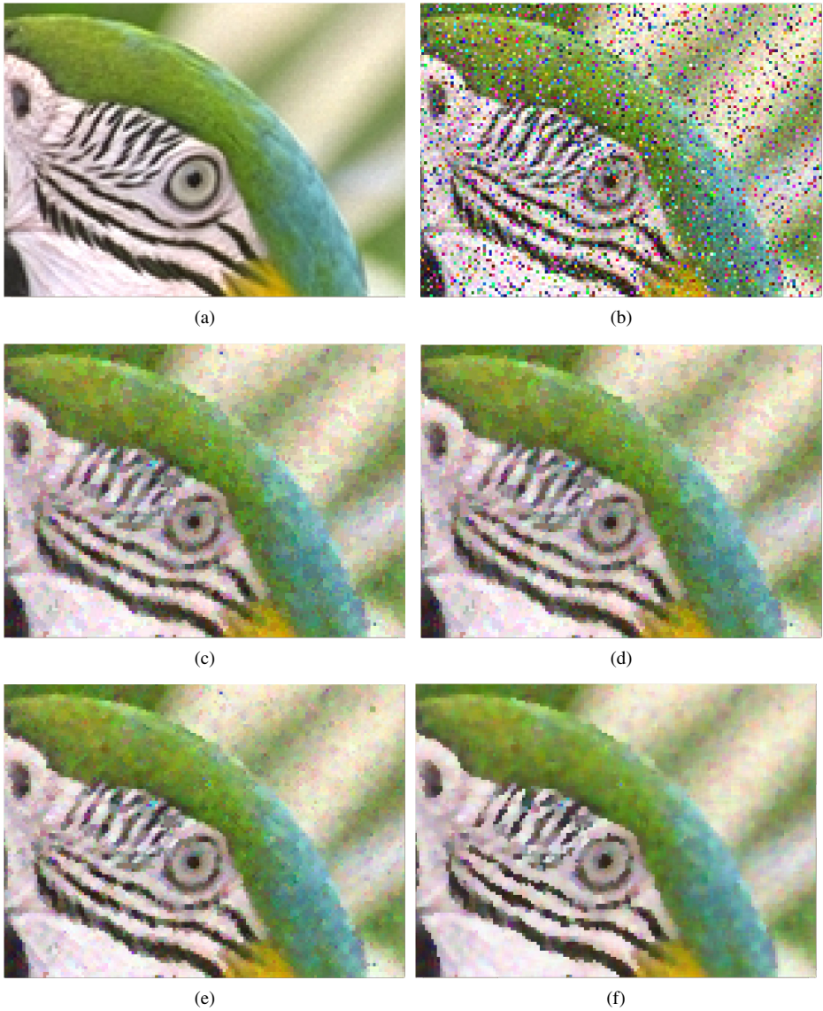
Fig. 5. Filter outputs of the (a) Parrots image, (b) image corrupted with p = 0.2 impulse and \sigma = 20 Gaussian noise and outputs from (c) VM filter (d) FROD filter (e) FPG filter (f) DENS filter
