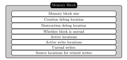
Fig. 4. Structure of a Memory Block
