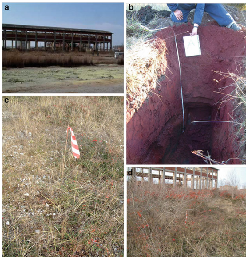
Fig. 8.1 Polluted site at Torviscosa (Udine, NE Italy). (a) Yellow deposit of sulphur on soil surface near abandoned factory. (b) Exploratory ditch (1.5 m) for studying soil/pyrite stratigraphy. (c) Detail of gravelly capping soil with aged spontaneous vegetation (in winter). (d) Dense vegetation of Pyracantha coccinea M.J. Roemer (in winter) close to old factory
