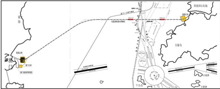
Fig. 116.3 General layout of the Hong Kong-Zhuhai-Macao bridge
