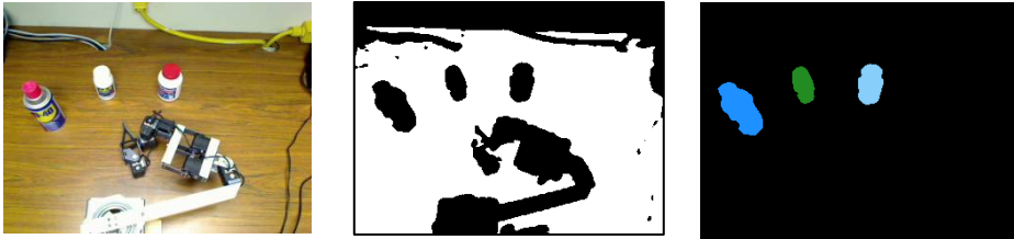
Fig. 2. The system uses a simplified object finding routine. The steps of this process are to take the input image (left) and enhance its color, find a uniform description for the majority of the area (middle), then identify isolated, non-table regions (right).
