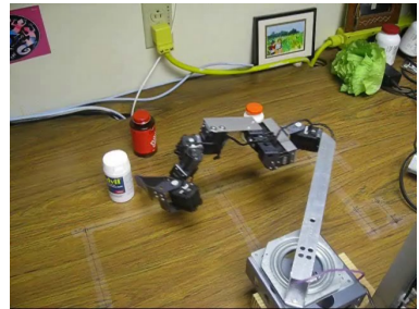
Fig. 9. As this transcript of one of the video demos [1] shows, the robot can be taught a new verb by simply walking it through the appropriate steps
