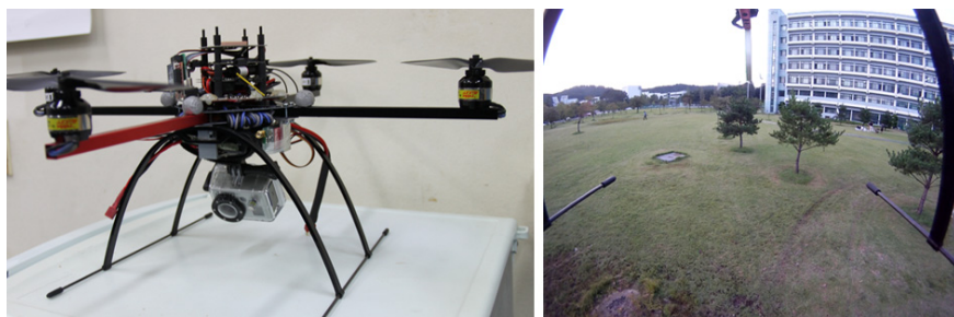
Fig. 2. A multi-rotor platform equipped with a single camera (left) and an image taken by the platform during manual flight (right)
