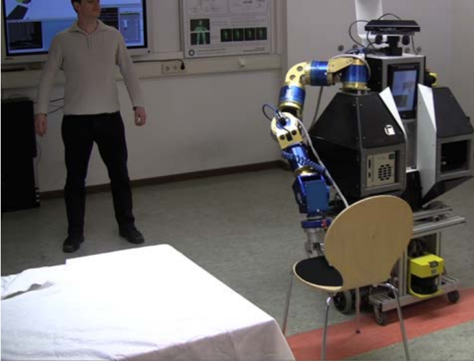
Fig. 5. Execution snapshot. Interacting human on the left, robot performing the robot role. Manipulation actions are executed using parameterized motion and grasp planning with online object localization.
