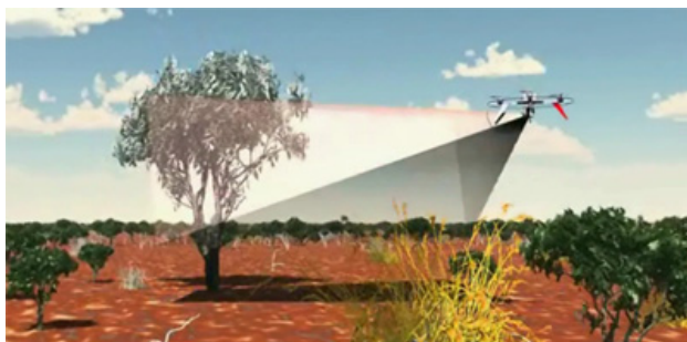
Fig. 1. Image acquisition task for 3D tree model reconstruction using a multi-rotor UAV
