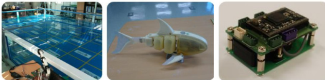
Fig. 1. Water tank and robotic fish and DSP module with MEMS IMU (3DM-GX3-35)
