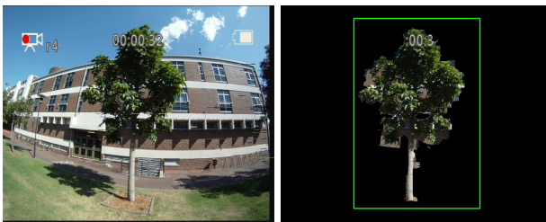
Fig. 4. Image segmentation. An input image (left) is segmented into the tree and the background (right) by using an image segmentation algorithm. The extracted silhouette is used to construct the volumetric model of the object.
