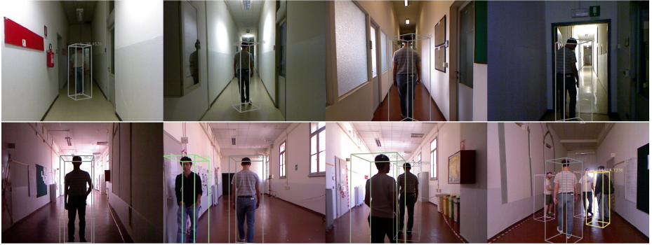
Fig. 7. People following test. First row: examples of tracked frames while a person is robustly followed along a narrow corridor with many lighting changes. Second row: other examples of correctly tracked frames when other people are present in the scene.
