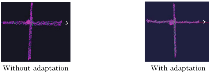
Fig. 6. Effect in the adaptation of the consistency. The distance from the sensor to the features increases in the direction of the arrow. Notice that the dispersion of the position increases with the distance to the sensor when no adaptive consistency is used
