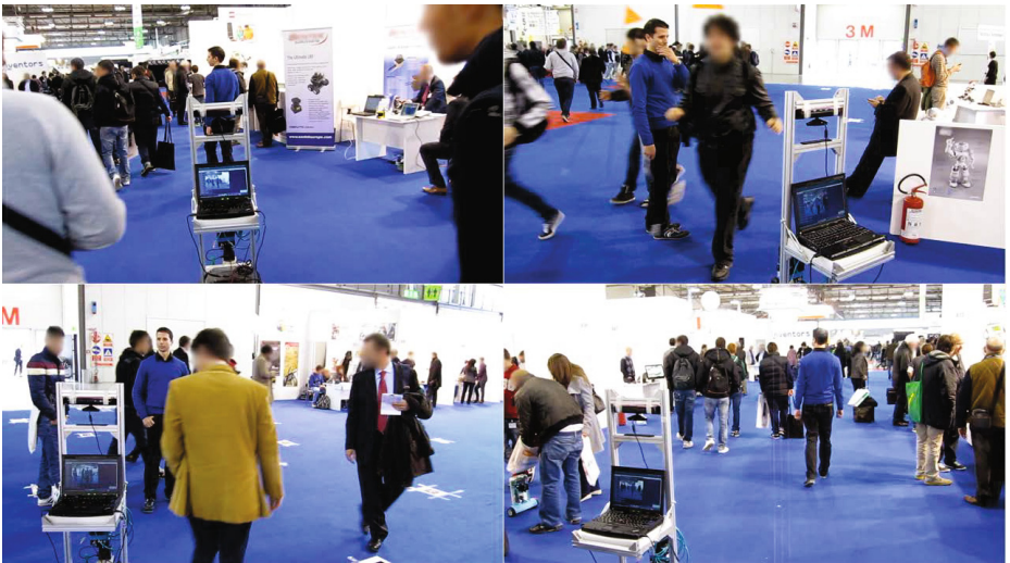
Fig. 8. Sample images of our mobile robot following the person with the blue sweater within a crowded environment. It is worth to notice that the sweater has the same color of the carpet on the floor.
