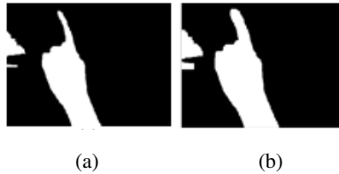
Fig. 5. (a) Erosion result (b) Dilation result
