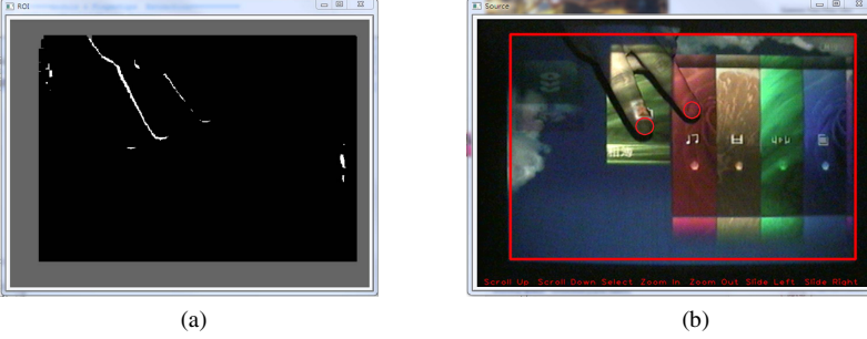
Fig. 4. (a) Shadow detection (b) Fingertips Extraction
