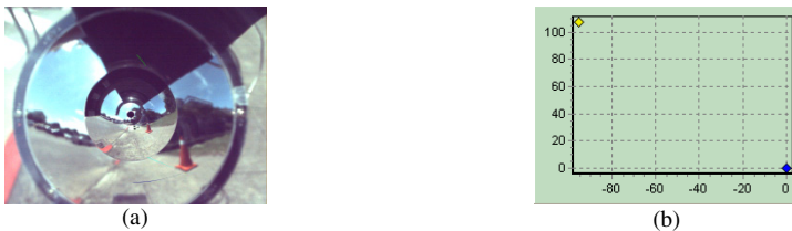
Fig. 18. Result of traffic cone localization. (a) Result of extracting L_X , L_Y , and L_Z lines of traffic cone (b) Computed position of traffic cone (yellow spot) with respect to vehicle.
