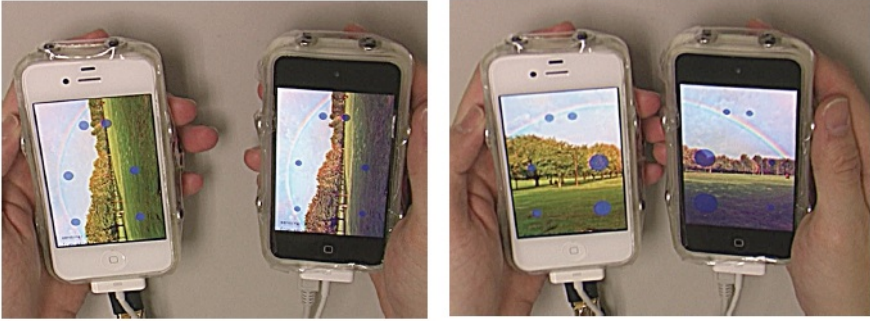
Fig. 5. Two phones with MagMobile module (left). They can detect magnetic change in short distance and stitch screens (right). Each blue dot on the screens represents magnetic force sensed by a sensor unit.
