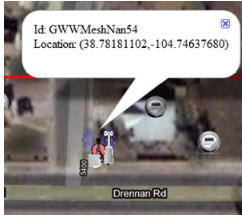
Fig. 2. Using SG-WIP tool for planning the antennae position. A WiMAX/Wi-Fi gateway was placed on a streetlight pole.
