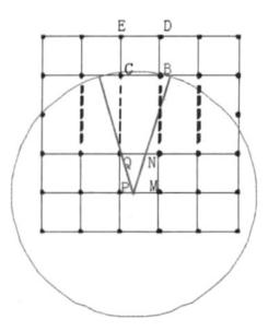
y + n + 1), reader B, C, D, E four-point detection status of (Sb and Sc, Sd, Se), the change process (false, false, false, false)  $\rightarrow$  (true, false, false, false)  $\rightarrow$  (true, true, false, false), you can determine reader in regional PMNQ, and even if in this process, the reader reads *B* and *C* in the same horizontal position, but also to determine the reader in the Regional PMNQ its error range in the M point, the error is 0, that is, to achieve accurate positioning.
