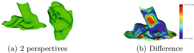
Fig. 2. Typical example of an ear impression from two perspectives and an example of the difference map between an open and a closed mouth impression
