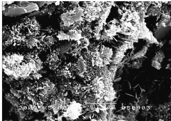
Fig. 40.13 SEM image ( \times 5000 ) of silica sand cement paste maintained at room temperature for 28 days
