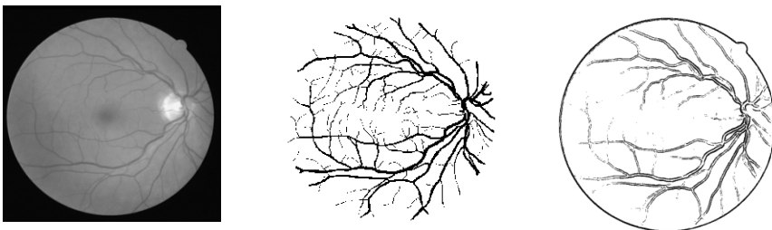
Fig. 2. Retinal fundus image 2 (a), Ground truth (b) , PSO based multilevel Tsallis thresholding (c)
