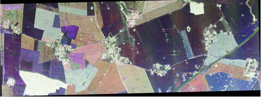
SAR Images, Interpretation of, Fig. 7 False color image obtained by performing a Pauli decomposition on the polarimetric SAR image of an agricultural area
