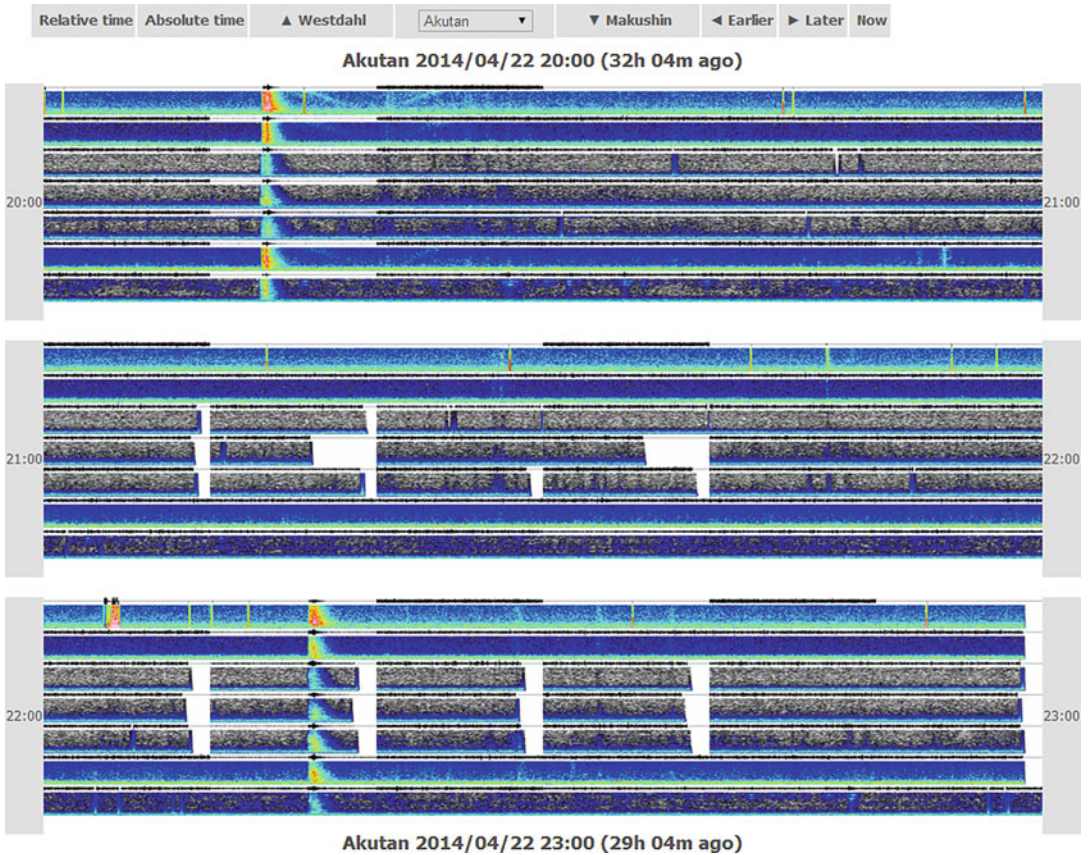
Seismic Monitoring of Volcanoes, Fig. 5 A spectrogram mosaic, part of the same application shown in Fig. 4. Three hours of data are shown. Regional earthquakes are
