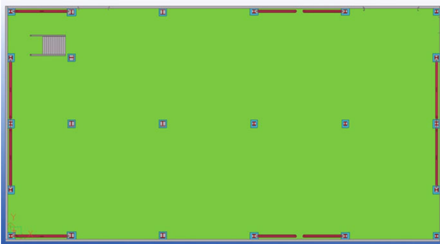
Seismic Analysis of Steel Buildings: Numerical Modeling, Fig. 5 Plan view of prototype building’s 3D model above foundation level
