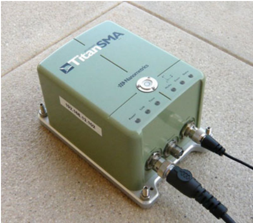
Seismic Accelerometers, Fig. 16 Nanometrics Titan accelerograph. Its size is approximately 18 x 12 x 10 cm
