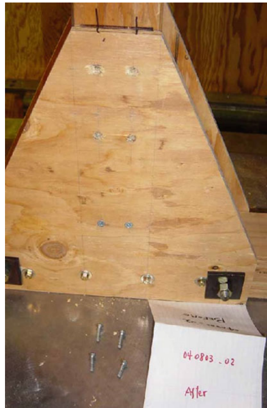
Seismic Response Prediction of Degrading Structures, Fig. 13 Failure configuration of T -connection under excitation A over 1,000 s
