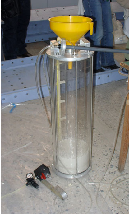
Strengthening Techniques: Masonry and Heritage Structures, Fig. 11 Device for mechanical mixing of the grout before application
