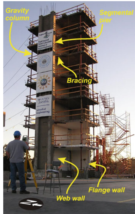
System and Damage Identification of Civil Structures, Fig. 2 Seven-story shear wall test structure
