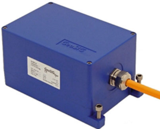
Seismic Accelerometers, Fig. 17 FBA with MEMS technology AC-43 from GeoSIG. It weights 2 kg and its size is 19 x 11 x 9 cm (Figure from GeoSIG ( www.geosig.com/AC-4x-id10357.html ))
