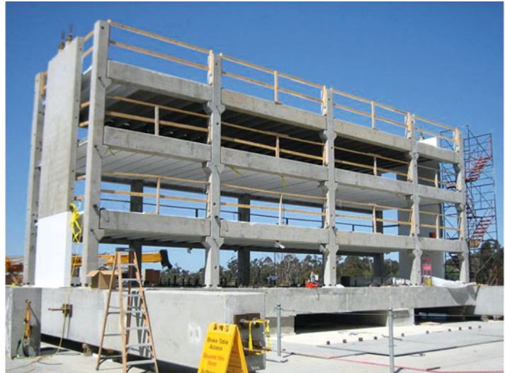
System and Damage Identification of Civil Structures, Fig. 3 Front view ( left ) and side view of the three-story reinforced concrete frame with masonry infilled walls ( right )
