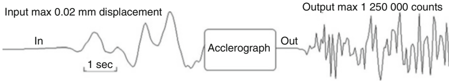
Seismic Instrument Response, Correction for, Fig. 1 The input is the ground moving with a maximum displacement 0.02 mm. This “signal” goes through an
