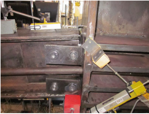
Steel Posttensioned Connections with Web Hourglass Pins: Toward Earthquake Resilient Steel Structures, Fig. 13 Gap opening at 6 % imposed drift of the SC-WHP1 specimen
