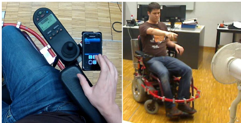
Fig. 1. Interaction paradigms: on the left using the touch screen integrated in the smartphone and on the right through natural deictic gesture
