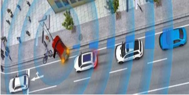
Fig. 2. A VANET preventing a multi-vehicle collision [17]
