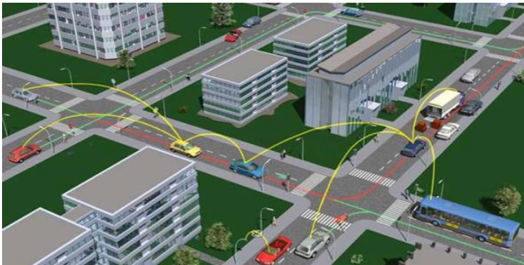
Fig. 1. A VANET in a city scenario. Vehicles are warned of the truck blocking the road and find alternate routes [17].
