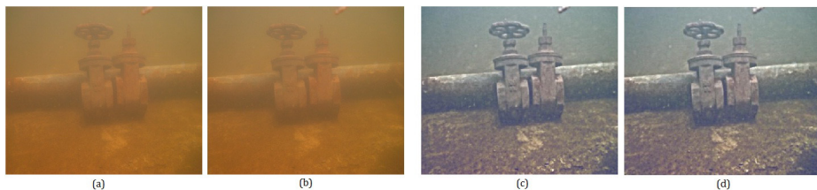
Fig. 2. Data Set2: Captured Underwater video frames (a) Frame 1 and (b) Frame 20 ; After color-correction (c) Frame 1 and (d) Frame 20
