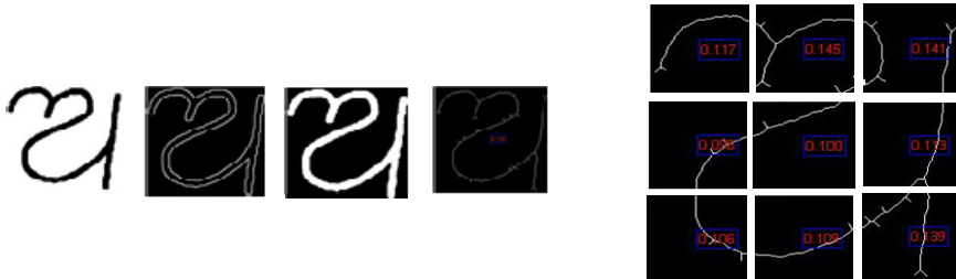
Fig. 5. The Character (A) and its 9 equal zones showing standard deviation values
