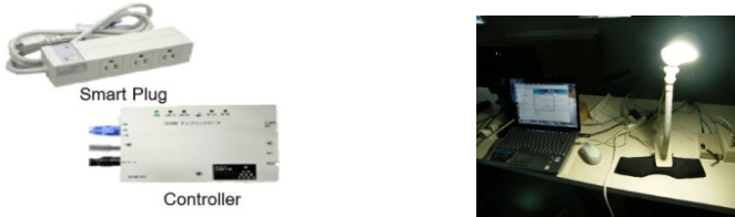
Fig. 4. Implementation of smart plug to control home appliances, e.g., a lamp
