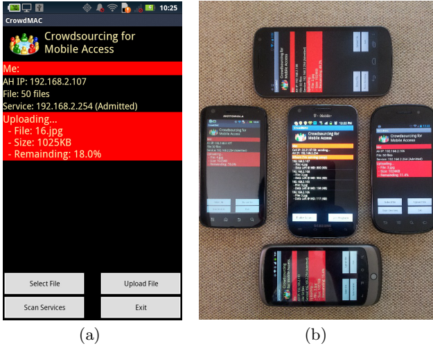
Fig. 3. Our Android based testbed: (a) a screenshot of our system on a mobile device and (b) an experiment with 5 different types of mobile phones
