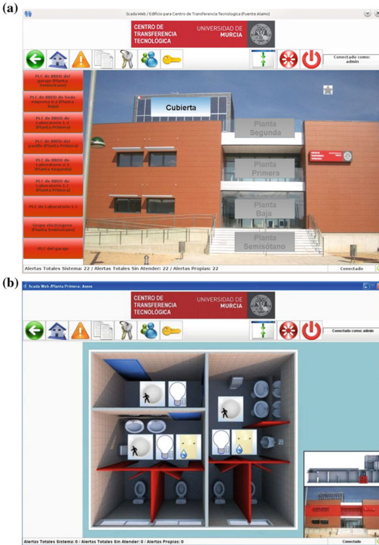
Fig. 7 JNLP application with 3D HMI for local/remote management through the SCADA-web access. a Overall building view. b Monitoring the bathroom of the 1st floor
