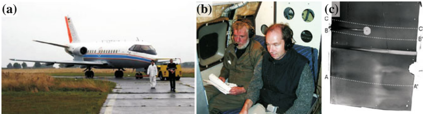
Fig. 2.5 DLR's VFW 614 ATTAS (a), scientists during flight test (b) and recorded PSP pressure distribution (c)
