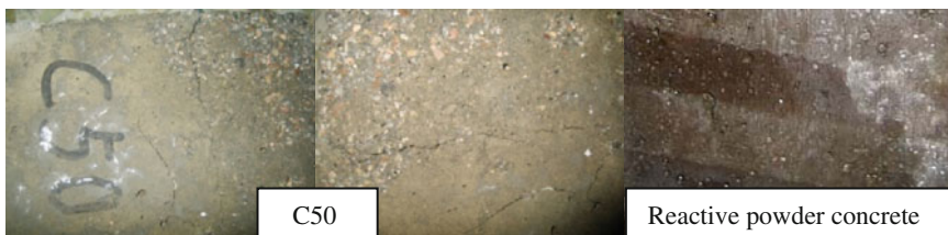
Fig. 116.2 The surface morphology of specimens after freeze-thaw cycles
