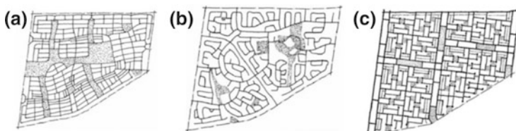
Fig. 18.1 (a) Traditional squares grids (b) traditional ended type (c) fused grid structure
