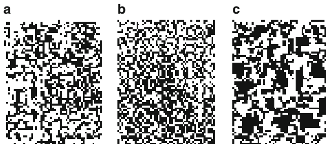
Fig. 4.19 Micro-heterogeneities in glasses modeled by distributions of black and white squares according to a classical picture given by Laves: (a) system with a relatively slight aggregation of white squares, (b) statistical random distribution, (c) pronounced clustering (See Vogel (1979) [889])
