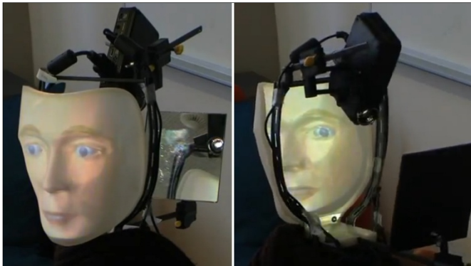
Fig. 8. A front and back view of the mask and the rig of Furhat
