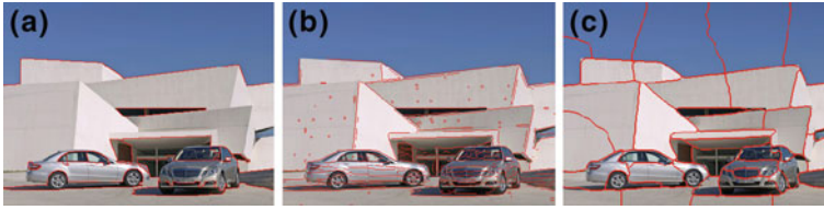
Fig. 57.1 Segmentation results with four classical algorithms. a watershed. b Meanshift. c N-cuts
