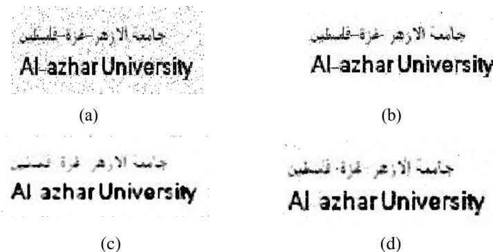
Fig. 6. Restoration of 5% corrupted machine-printed document image with random valued impulse noise: (a) Corrupted version (b) New method, (c) ACWMF[17], (d) TSMF[18]
