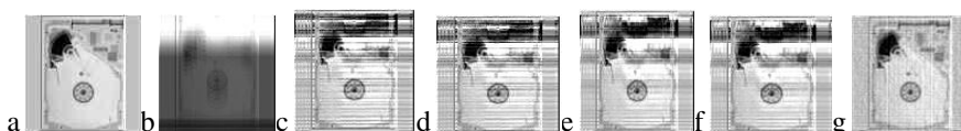
Fig. 10. a) Original image of computer hard disk, b)blurred image, c) TSVD, d) Tikhonov regularization, e) Tikhonov (sobolev), f) TV solved by split Bregman method, g) Hybrid BFO-PSO
