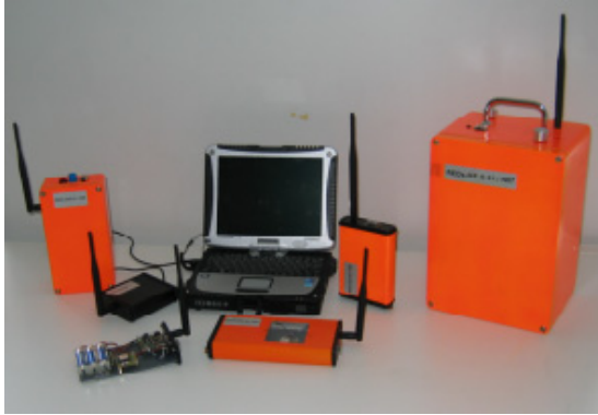
Fig. 1 REDs probes and controller, from left to right. Back: audio probe, gateway, REDs controller, accelerometer, gas sensor system. Front: GPS node (open and closed).
