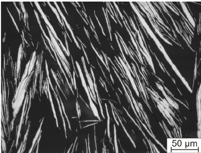
Fig. 1 Optical micrograph of milled AA-2017 without reinforcements and 0.5 wt.-% stearic acid after 4 h of milling time
