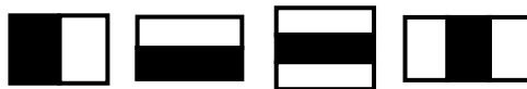
Fig. 1. Four kinds of features used in our method, containing two or three rectangles
