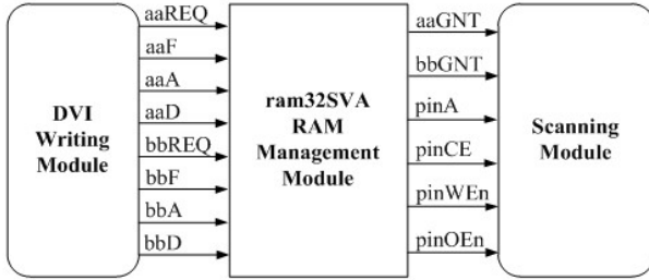
Fig. 3. Principle Scheme of ram32SVA – RAM Management Module
