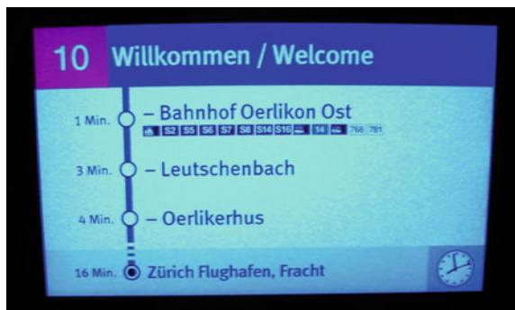
Fig. 1 Public screen inside a tram in Zurich, Switzerland showing time estimates for the next three stops and the final destination, as well as connecting lines at the upcoming train station Bahnhof Oerlikon Ost
