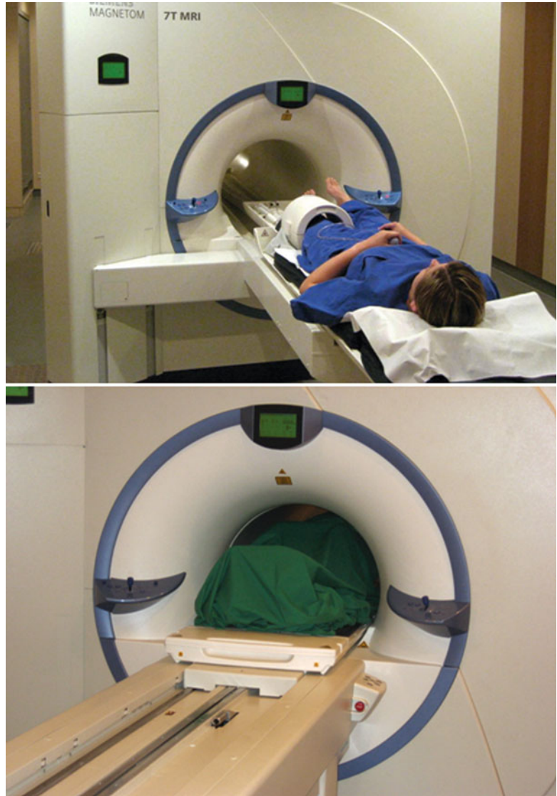
Fig. 5.1 7-T MR scanner with a bore of 60 cm and a length of 3.50 m. The MR is surrounded by 425 tonnes of steel. The upper figure shows a person before positioned feet first into the scanner. The lower figure shows a person head first in the scanner with the head in the isocentre, the feet covered with a sheet. The scanner used here is located at the Erwin L. Hahn Institut, Essen, Germany
