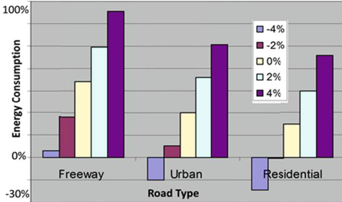
Fig. 8. Comparison of the effect of road gradient on the three types of roads: freeway, urban highway and residential road
