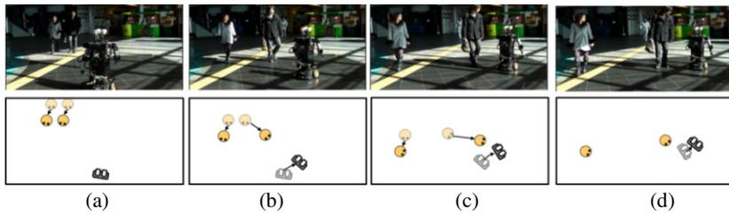
Fig. 11. The robot safely avoids an approaching pedestrian
