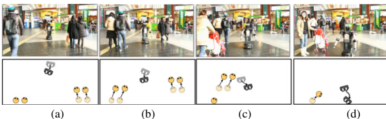
Fig. 10. The robot safely navigates through pedestrians in the mall
