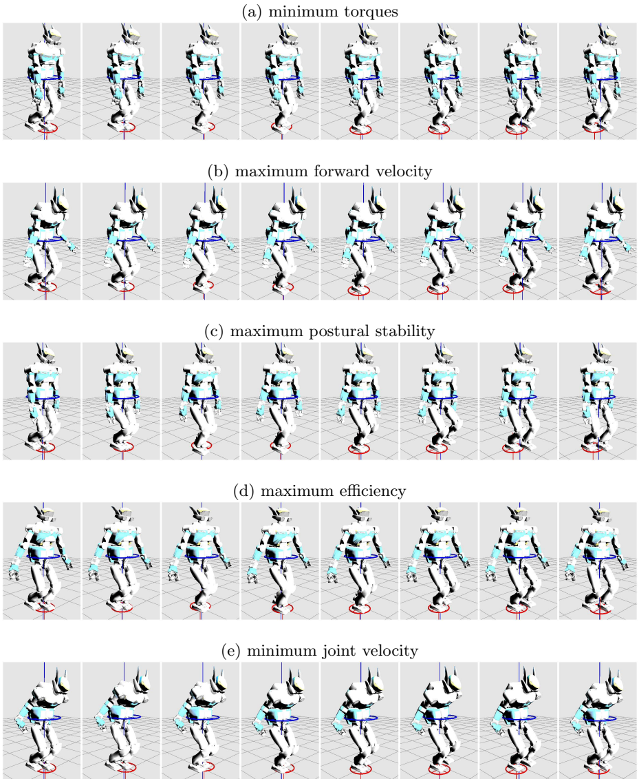
Fig. 2. Walking sequences for HRP-2 with free foot placement and constrained ZMP for different objective functions (center of circle on the floor represents ZMP, center of circle near pelvis shows CoM)
