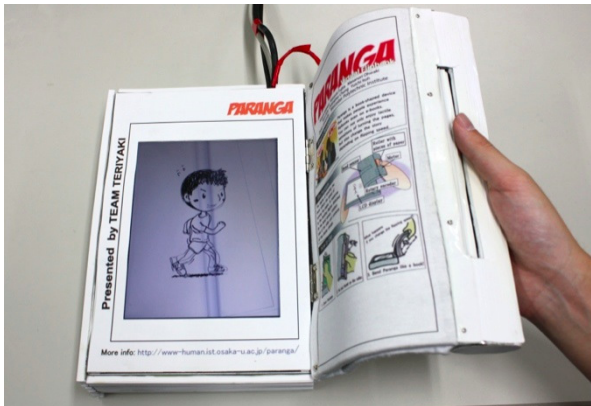
Fig. 1. Overview of Paranga Paranga is a book-shaped device that has a rotatable roller to provide a user with the tactile sensations of page turning.
