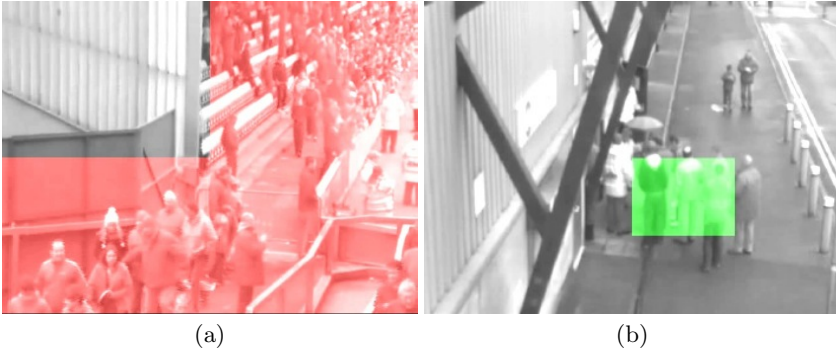
Fig. 1. Example of classification output, for image divided into 4 (a) and 16 (b) regions. The color rectangles are superimposed on crowd detection output; colors indicate density: red stands for ‘high’ class, green for ‘mid’ class.
