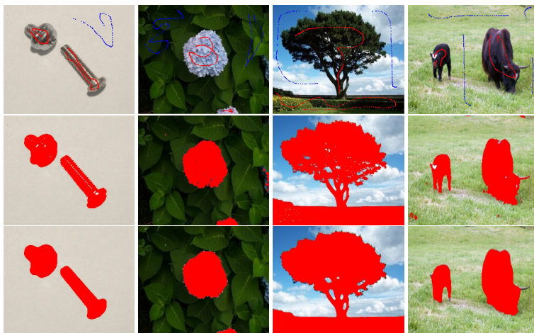
Fig. 2. Experimental results from the Berkeley Segmentation Dataset. Each column displays one scene. The first row is the input image with user label, where red denotes foreground pixels and blue. The second row is the segmentation results using graph cuts, and our results are shown in the third row.
