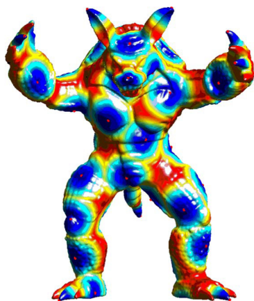
Fig. 2. Assignment of Centers: Using geodesic farthest point sampling on the topology model, 50 points are uniformly positioned on the Armadillo 3D mesh
