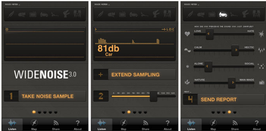
Fig. 1 EveryAware WideNoise start screen, decibel prediction screen and qualitative rating of the noise
