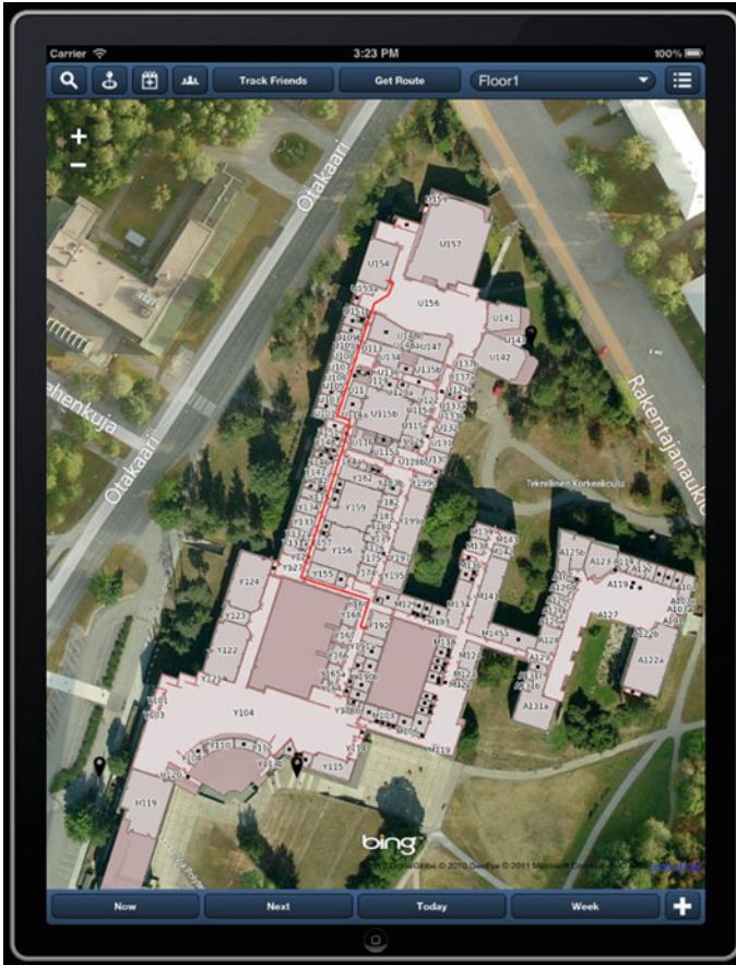
Fig. 1 View of the prototype application that contains both indoor and outdoor map, and a shortest route
