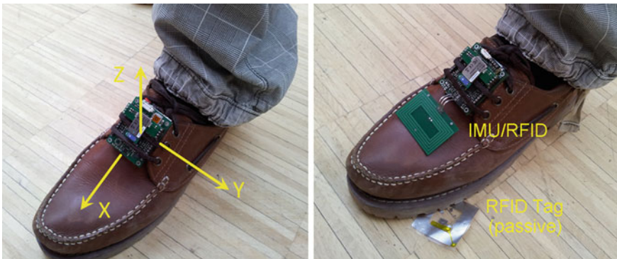
Fig. 5 Custom IMU mounted on a foot ( left ) with body coordinate frame and IMU augmented with RFID reader antenna and tag beneath the foot ( right )
