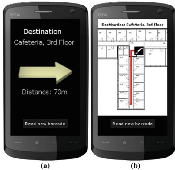
Fig. 1 Simple navigation instruction (a) and map overview (b) [both from Ruppel and Gschwandtner (2009)]
