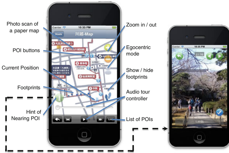
Fig. 12 Main interface of the prototype. The map is provided as a paper map by SEIBU Railway Co., Ltd. for a walking tour event around center of Kawagoe area, Saitama Prefecture in Japan on May 6th, 2012. The number of participants is about two thousands. We have created a location-based service on iPhone using the paper map of Kawagoe as a base map and experienced on the same time
