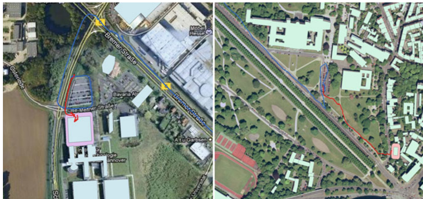
Fig. 8 Optimized route planning scenarios showing precise classification and extraction of parking place associated with desired address avoiding detour and loss of valuable time: car trace in blue, walking trace in red, destination in pink polygon
