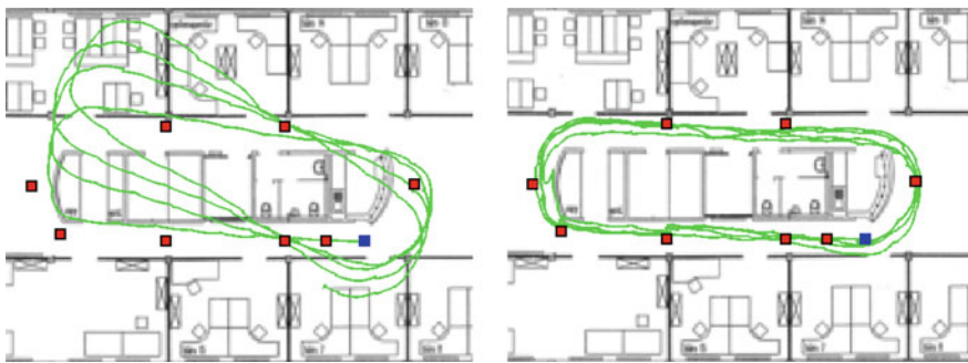
Fig. 14 Comparison of pure inertial localization ( left ) and approach augmented with RFID measurements ( right ) in single floor scenario. Red squares mark the position of RFID tags while the blue square denote the start of the walking trajectory
