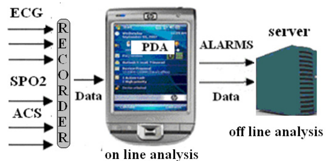
Fig. 1 Architecture of system.
