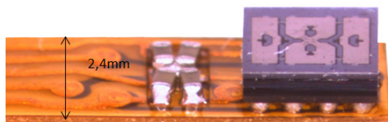
Fig. 4 The integrated design of cable and substrate.
