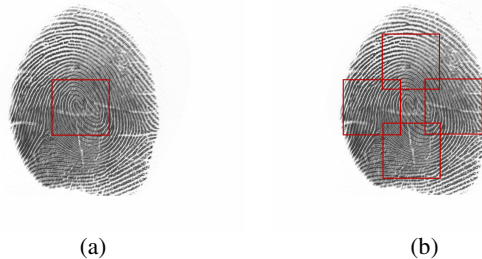
Fig. 1. ROI positions. (a) Baseline ROI. (b) Wrong locations: up, down, left, right.
