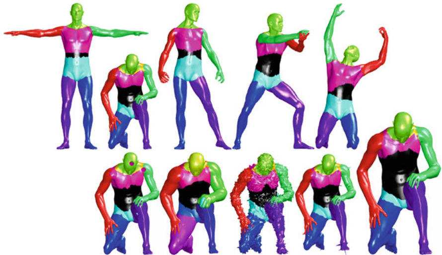
Fig. 8.2 Maximally stable regions detected on shapes from the SHREC'10 dataset using the vertex weight h_t(v, v) with t = 2,048 . First row : different approximate isometries of the human shape. Second row : different transformations ( left-to-right ): holes, localscale, noise, shotnoise and scale
