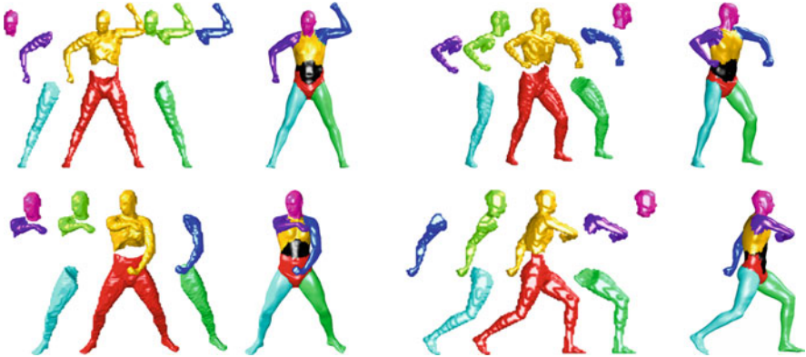
Fig. 8.7 Stable volumetric regions detected on the SCAPE data [1]. Shown are volumetric regions ( first and third columns ) and their projections onto the boundary surface ( second and fourth columns ). Corresponding regions are denoted with like colors. The detected components are invariant to isometric deformations of the volume
