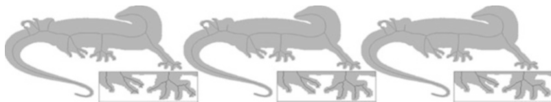
Fig. 4.4 The lizard shape is an example of skeletons that are similar in size and exactness of reconstruction, but vary in complexity. FOAT ( middle ) and MDT ( right ) feature less branches in the small details of the lizard such as in its toes. FOT ( left ) produces additional branches, in particular for jagged edges that result from the discretisation of the shape boundary, as it strives in this example for a very exact representation
