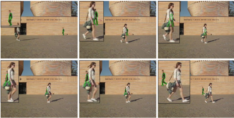
Fig. 18.4 Results of our algorithm on walking man sequence (173 frames) with full occlusion (walking woman hides the target). The algorithm automatically switches from on-line learning (frame 95) to PCA representation as soon as occlusion is detected (frames: 35,100,101,103,104,109)
