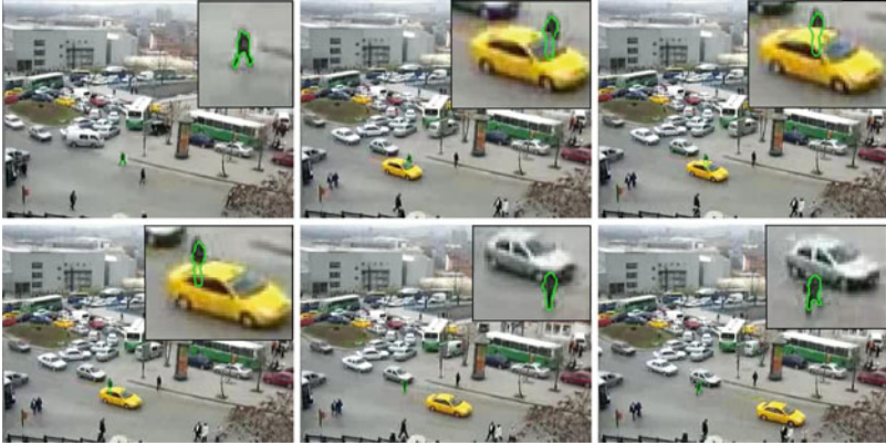
Fig. 18.3 Results of our algorithm on walking man sequence (200 frames) with partial traffic occlusions ( yellow and silver car ). The algorithm automatically switches from on-line learning (frame 60) to PCA representation as soon as occlusion is detected (frames: 11,66,68,70,77,84)
