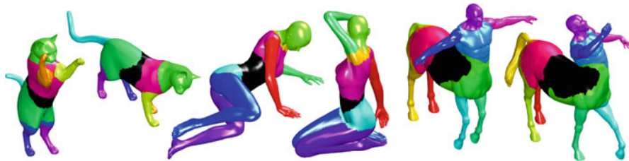
Fig. 8.1 Maximally stable regions detected on different shapes from the TOSCA dataset. Note the invariance of the regions to strong non-rigid deformations. Also observe the similarity of the regions detected on the female shape and the upper half of the centaur (compare to the male shape from Fig. 8.2). Regions were detected using h_t(v, v) as vertex weight function, with t = 2,048
