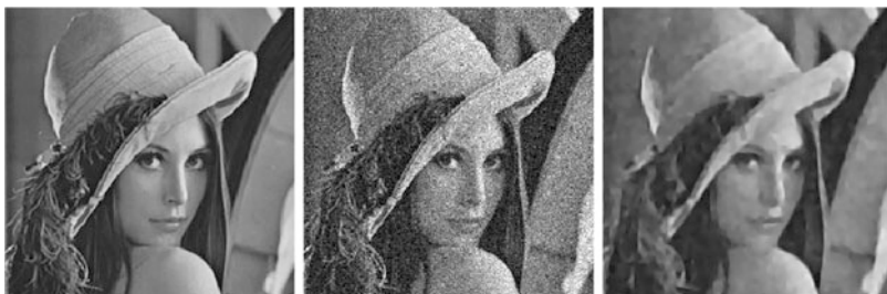
Fig. 9.10 Original, noisy ( v = 25 ) and filtered image by AMSS ( C = 0.02, s = 1, \Delta x = 1, \Delta t = 0.25, \rho = (\Delta t)^{1/6}, N = 10 )
