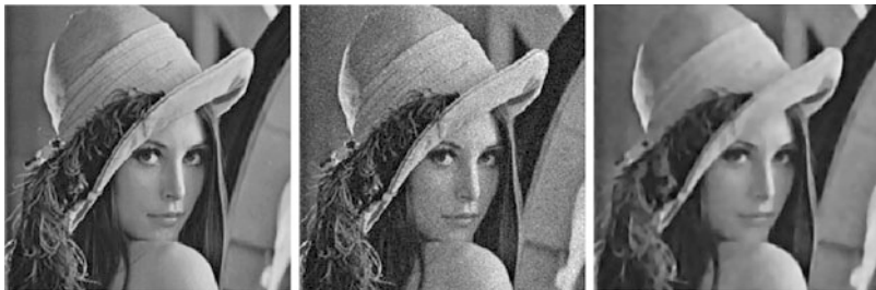
Fig. 9.9 Original, noisy ( v = 12 ) and filtered image by AMSS ( C = 0.02, s = 1, \Delta x = 1, \Delta t = 0.2, \rho = (\Delta t)^{1/6}, N = 10 )
