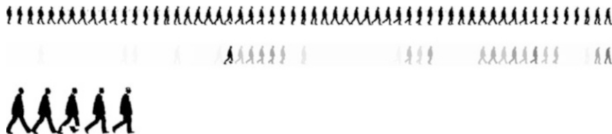
Fig. 7.7 The extracted silhouettes from a gait sequence are displayed (the first row ) and underneath is an intensity coding of each silhouette to show its degree of being an outlier ( dark means high likelihood). A magnified view of the most outlying silhouette and its neighbours is in the third row
