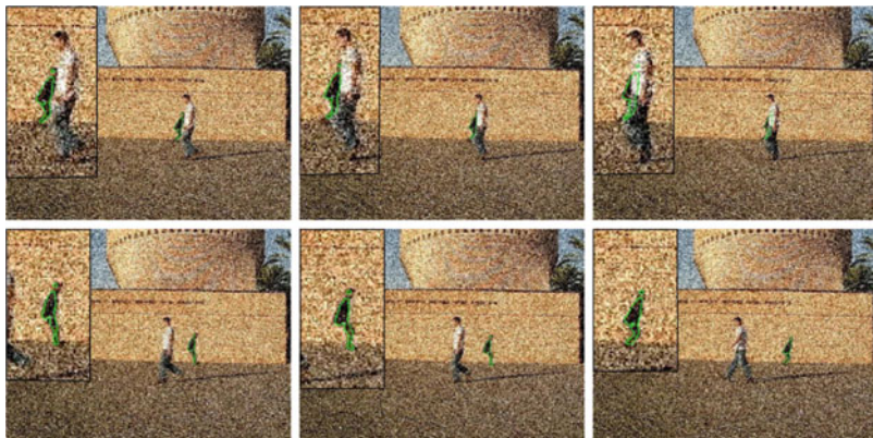
Fig. 18.7 Results of our algorithm on jumping man sequence with additive Gaussian noise ( \text{SNR} = 15 ) and full occlusion (walking man hides the target). Frames: 119,120,121,132,134,142
