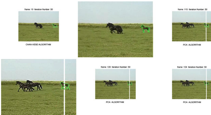
Fig. 18.6 Results of our algorithm on running horse sequence (290 frames) with one partially long period (synthetic) occlusion (20 frames with white label hides partially the target). We showed that our method was able to remain locked onto the target and illustrate the appropriate contours. Frames: 10,89,115,119,120,124
