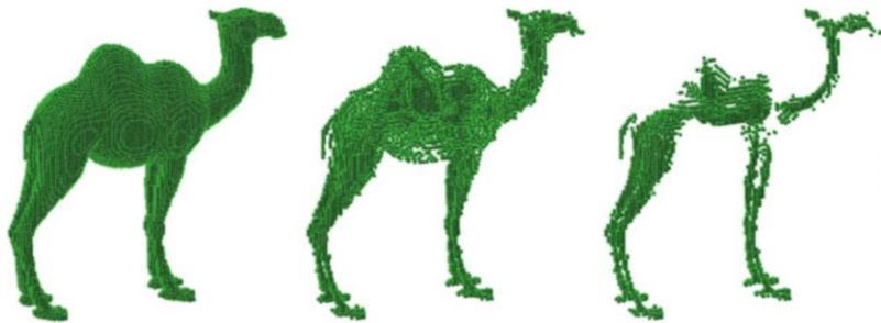
Fig. 6.1 From left to right , a 3D object X , the set of centers of maximal balls CMB(X) , and the set of relevant centers of maximal balls RCMB(X)
